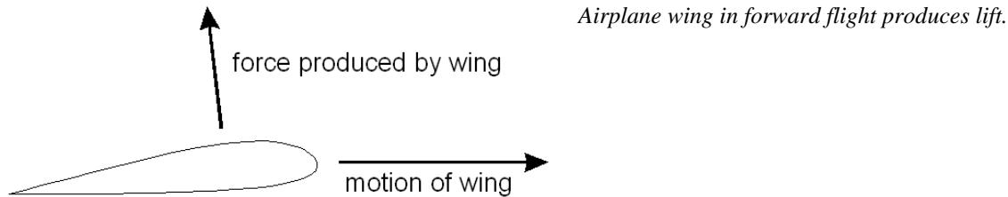
Notice that the force produced is not perfectly straight up. There is some "drag" which tries to hold the airplane back. It is counteracted by the propeller.
