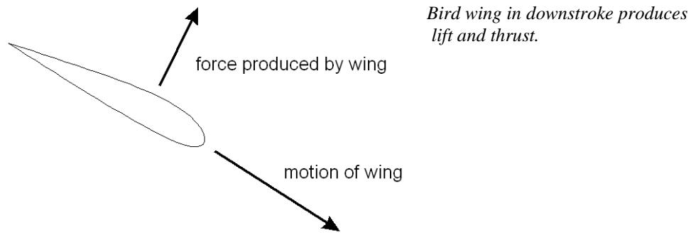
The downstroke is what keeps the bird going. The wing acts just like an airplane wing, but since it's moving at an angle, the force it produces is at an angle too. The wing produces lift, to keep the bird up in the air, and it also produces thrust, to keep the bird moving forward. That's why birds don't need propellers.
